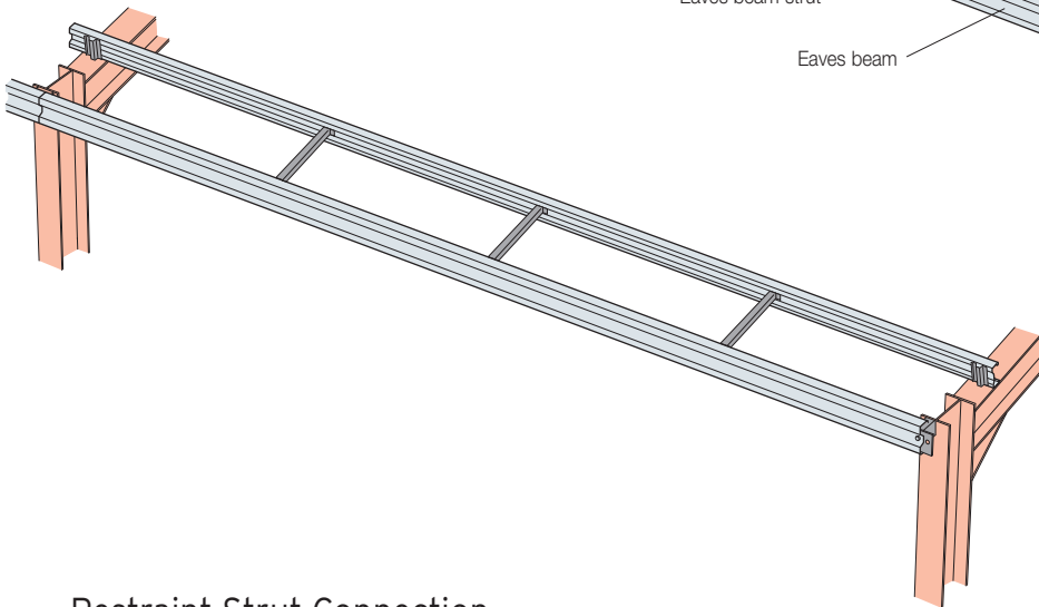
Bays over 9.5 - 12.0m Strut at 1/4 points
